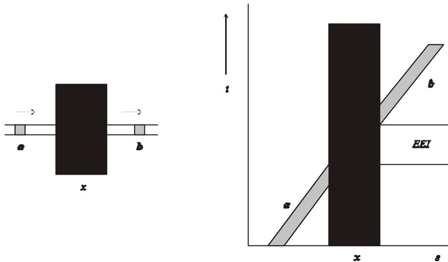
Figure. 1: Tunnel effect. At left its traditional sketching; at right a representation of it that can account even for the dimension of time. ( $a$  = the first mobile;  $b$  = the second mobile;  $x$  = a screen covering the trajectory of the two mobiles;  $t$  = axis of physical time;  $s$  = one-dimensional representation of frontoparallel plane;  $EEI$  = entry-exit interval of time, from the disappearing of the first mobile to the appearance of the second mobile.)
